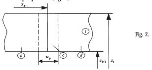
In the areas *s* and *d* we will consider that the elastic properties are constant, variations existing only in the area c. In the hypothesis that the specific strain  $\varepsilon_{x}$  depends only of variable x than in the area s we have  $\tilde{a}$  specific strain of the following type:
